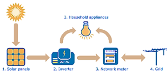
Figure 1: PV Systems in Energy Conversion
