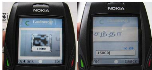
Figure 2: On the left, reviewing an entered value by focusing on a barcode. On the right, clicking brings up a prompt for editing the value. An audio prompt is also played.
