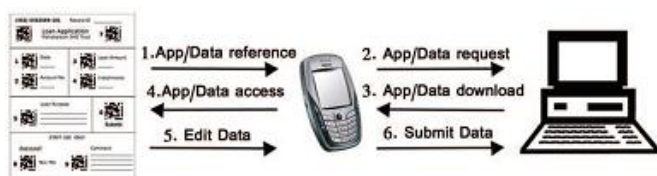
Figure 3: An example set of steps in accessing and using a CAM application. Except for steps 4-5, there can be arbitrary time and distance between each step, supporting an offline, asynchronous interaction model appropriate for rural areas.
