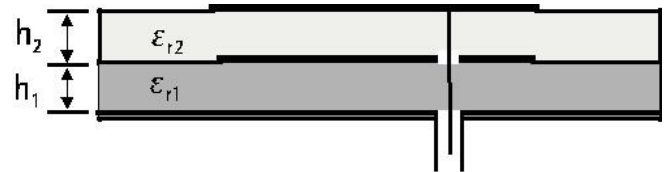
Figure: Electromagnetically coupled MSA with feed connected to top patch.
