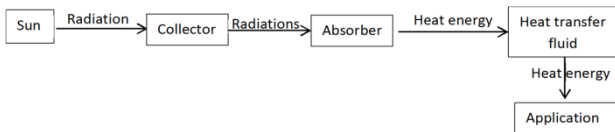
Fig.1.2. Working Principle of solar collector
