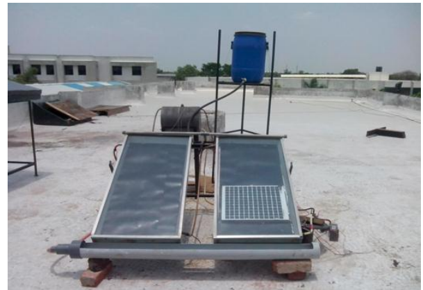
Figure 5.2 Solar PVT system set-up
