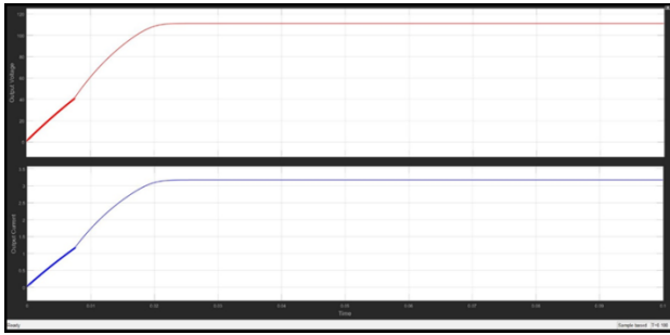
Fig 12- Solar PV Output Voltage and Current with droop control
