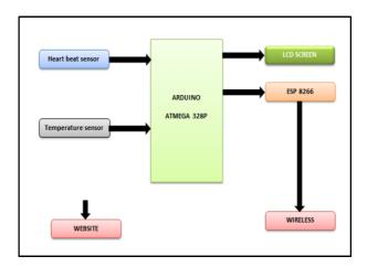
The given mapping diagram shows basic components used for the system functioning. Every component is linked to the arduino that is also referred to as the circuit's heart. The used coding can be used to help the component function rightly.
