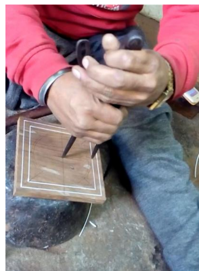
Fig -- Transferring the motif onto the wood with the help of Khaka
