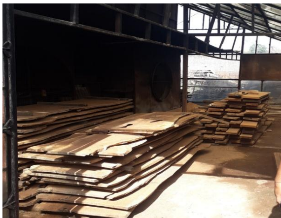
Wood is procured from the market and then seasoned in a special plant (Hoshiarpur)
