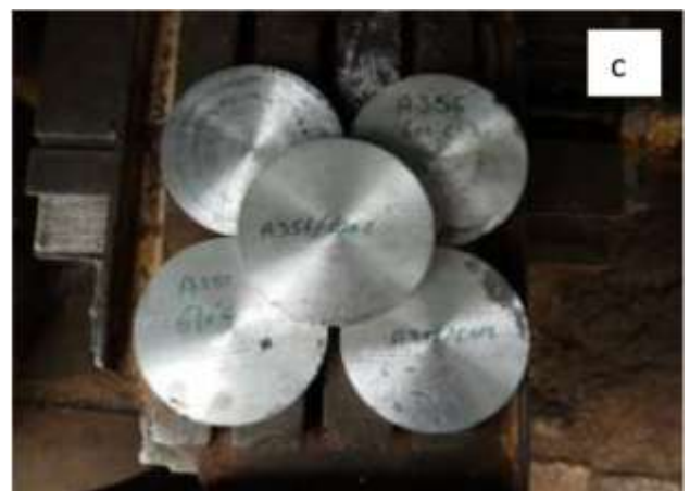
Fig. 3 (c) Thixocast Alloy after Machining (at diff. processing temperatures)
