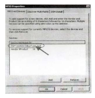
Step 12 - To add the second path to the iSCSI Target, open the iSCSI initiator Application and select the Target to use MPIO. Make sure it's connected.
