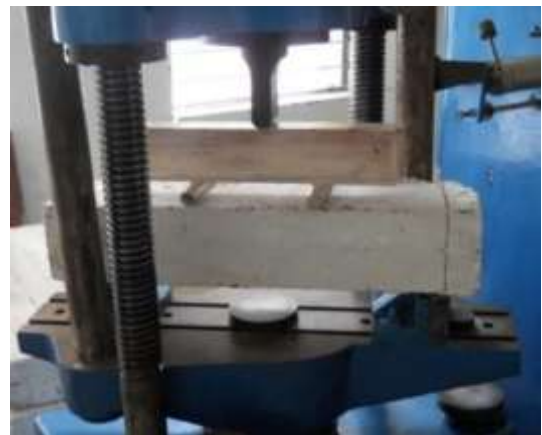
Image 6 : Testing of beams
