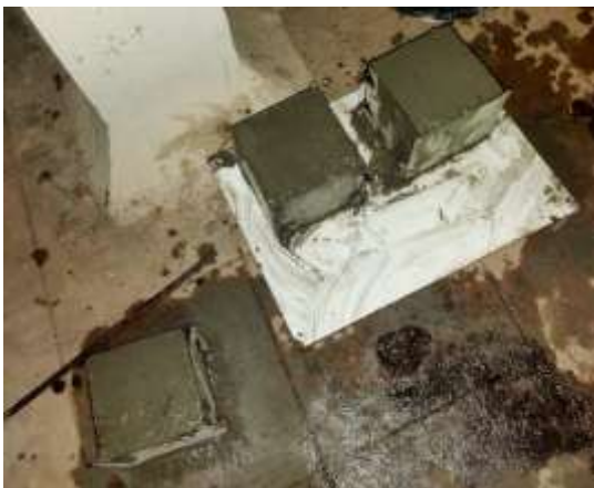
Image 3 : Placing of concrete in still position for 24 hours
