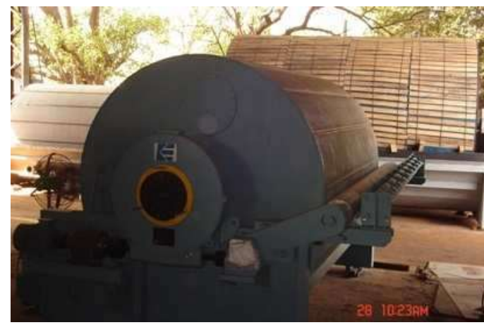
Fig.16: Rotary Vacuum Drum Filter Model for Experimentation
