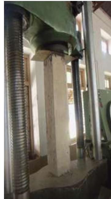
Figure 1: Failure Pattern of Unconfined Different Grades of Concrete Columns
