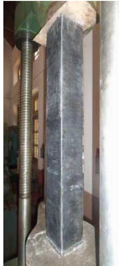
Figure 3: Failure Pattern of CFRP Strengthened Column with Different Layers
