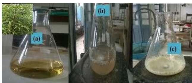
Figure 1 (a) Zanthoxylum armatum DC. leaf extract (inset plant image) (b) The solution mixture formed after addition of Zn(CH 3 COO) 2 .2H 2 O to the extract (c) Zanthoxylum armatum DC. leaf mediated ZnO NPs formed after addition of NaOH base to the solution mixture at 70 °C
