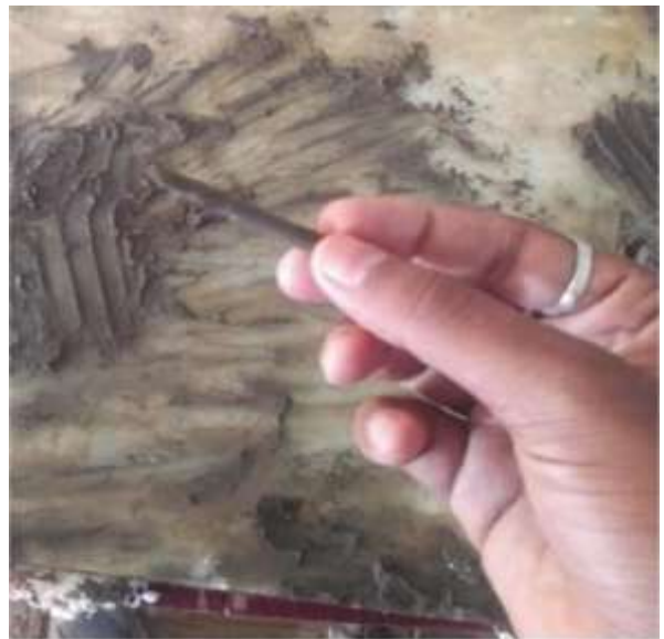
Figure 2: Liquid Limit and Plastic Limit Experimental Work
