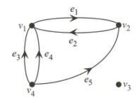
$$\mathbf{A} = \begin{pmatrix} e_1 & e_2 & e_3 & e_4 & e_5 \\ 1 & -1 & -1 & -1 & 0 \\ -1 & 1 & 0 & 0 & -1 \\ 0 & 0 & 0 & 0 & 0 \\ 0 & 0 & 1 & 1 & 1 \end{pmatrix} \begin{pmatrix} v_1 \\ v_2 \\ v_3 \\ v_4 \end{pmatrix}$$
