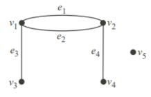
$$\mathbf{A} = \begin{pmatrix} e_1 & e_2 & e_3 & e_4 \\ 1 & 1 & 1 & 0 \\ 1 & 1 & 0 & 1 \\ 0 & 0 & 1 & 0 \\ 0 & 0 & 0 & 1 \\ 0 & 0 & 0 & 0 \end{pmatrix} \begin{pmatrix} v_1 \\ v_2 \\ v_3 \\ v_4 \\ v_5 \end{pmatrix}$$
