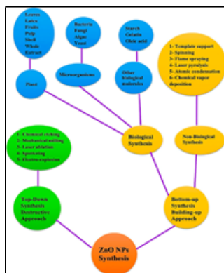
Figure 2: Standard procedures for the synthesis of nanoparticles of zinc oxide.
