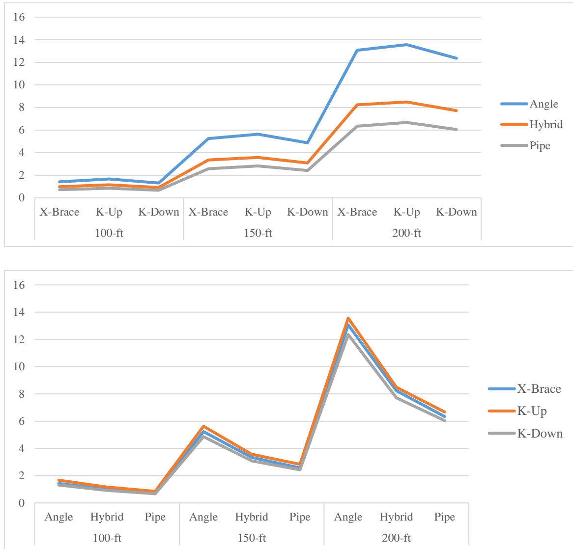
Figure 4: Maximum Horizontal Deflection For 3-Legged Tower
