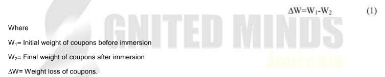
The percentage inhibition efficiency (%IE) was than calculated from the resulting weight loss data as follows:
