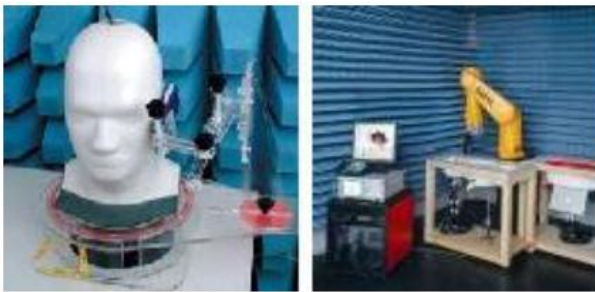
Figure 1. Different SAR measurement setups: (a) SAR measurement setup by Index SAR company, http://www.indexsar.com , and (b) SAR measurement setup (DASY5) by SPEAG, http://www.speag.com .
