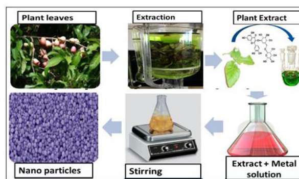
Figure 1.2: A schematic diagram of green synthesis of metal nanoparticles from plant extracts
