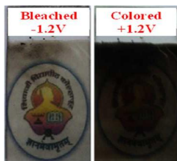
Figure.5.7: The photographs of a NiO film with a size of 2.5 \times 2.5 \text{ cm}^2 in colored (+1.2 V) and bleached (-1.2 V) states
