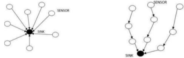
Figure 2: (a) Single-hop Communication and (b) Multi-hop Communication
