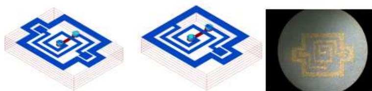
Fig.5 Square spiral inductor, 3D layouts with two port RF version left and grounded RF version middle (where blue is layer 6 metal and red is layer 5 metal) and two port RF version prototype (right)
