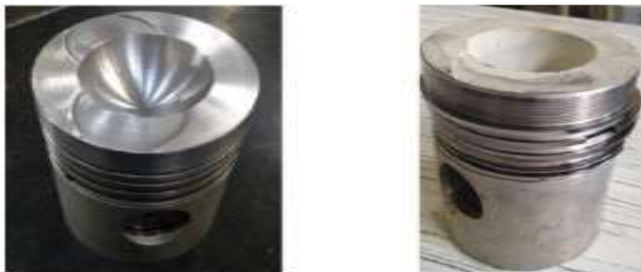
Figure 4: Uncoated and Coated piston Crowns
