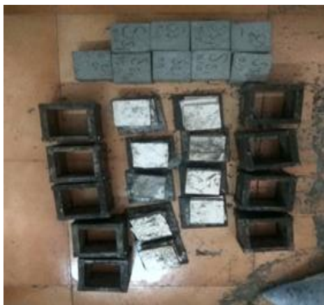
Fig .4.1: Abrasion Resistance Testing Moulds
