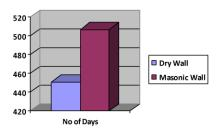
As per the simple calculation the construction time of the same structure of **56 days** will be save by using dry wall construction technique.
