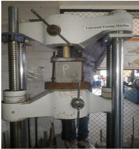
Figure 2 Assembly ready for pull-out test on cubes
