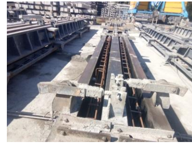
Beam Mould with Reinforcement
