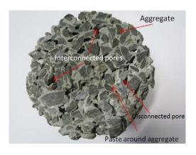
The Figure represents an example of PCPB cross-sectional area. It is a combination of good quality aggregate covered with adequate cementitious paste that leads to the formation of
