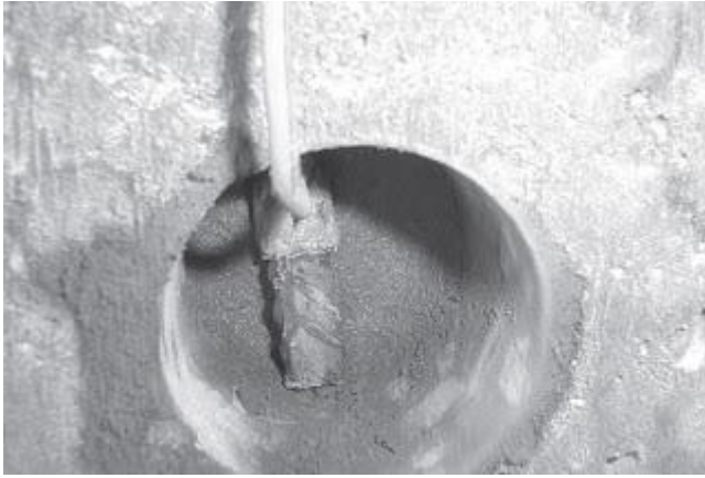
Fig. 4.2 Use of rebar probes
