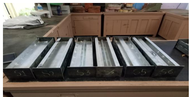
Test Sample of cold form of 450mm length
