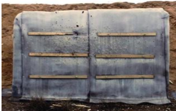
Figure 2:- CC as sandbag protection in defenses [Akhtar & Tyagi, 2015].
