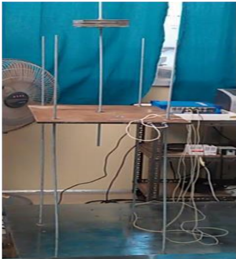
Single storey frame with TMD
