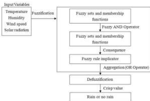
Figure 1. Fuzzy logic procedure of meteorological forecasting
