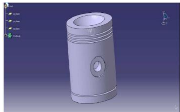
Fig.2 shows the completely modelled piston in CATIA.
