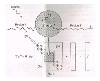
The GFB method consists of a generalization of the conventional FB approach which enhances the scope of application of the previous method to composite scattering problems as the one depicted in Fig. 1. The GFB formulation will be presented for a simple problem consisting of a sea surface containing only one obstacle (Fig. 1) The current is expressed as the sum of forward and backward contributions.
