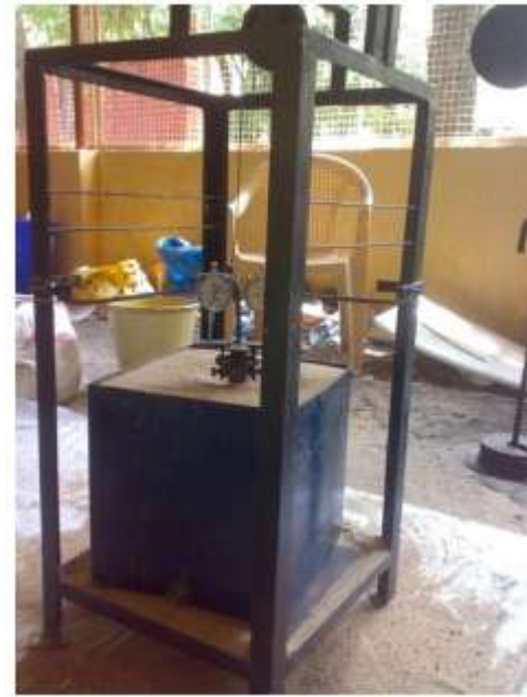
Figure 1.6 Model testing chamber with loading arrangement
