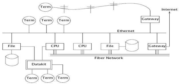
Figure. Structure of a large Plan 9 installation. CPU servers and file servers share fast local-area networks, while terminals use slower wider-area networks such as Ethernet, Datakit, or telephone lines to connect to them. Gateway machines, which are just CPU servers connected to multiple networks, allow machines on one network to see another.
