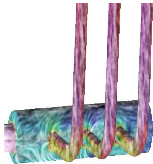
Figure: Visualization of flow on the surface of an intake manifold. The ideal intake manifold distributes flow evenly to the piston valves.
