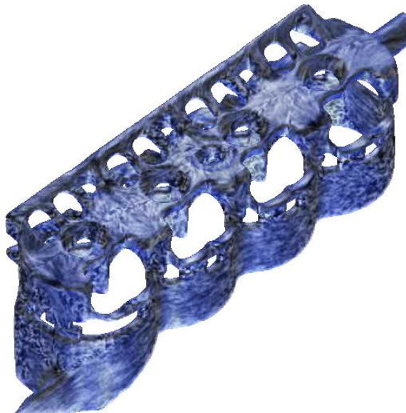
Figure : Visualization of flow at the complex surface of a cooling jacket -a composite of over 250,000 polygons.
