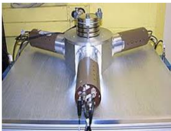
Figure 2: Three PMT in modern LSC-TDCR counters at 120° angle
