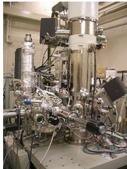
Scanning transmission electron microscope, used in metallography.
