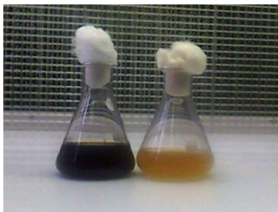
Figure 2: Microbially synthesized silver nanoparticles
