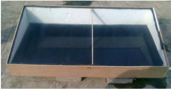
Fig.4. Working model of solar distillation system [4]
