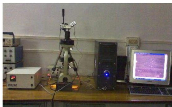
Figure 2. Optical transmittance measurement and texture study setup used in present work. The optical texture showing the texture clicked.
