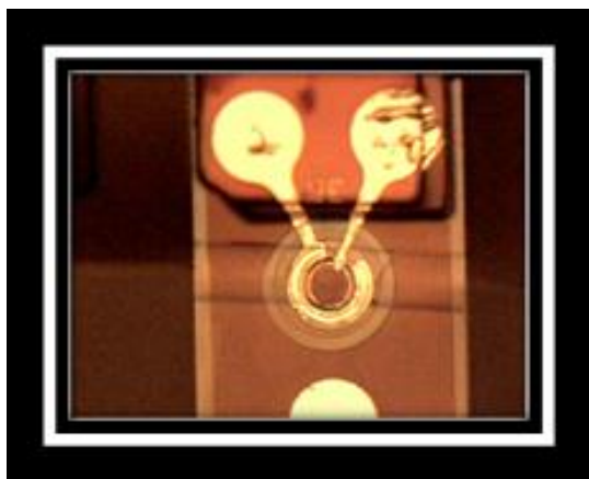
Figure 3- Embedded 10 Gbps Pin detectors in polymer waveguide on FR-4 board
