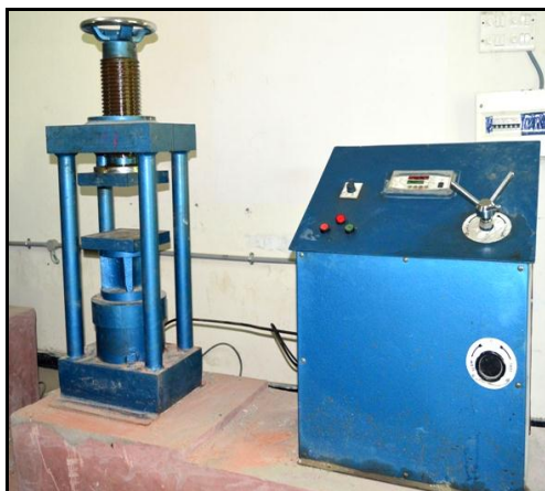
Fig. 4.1 Compressive Test machine
