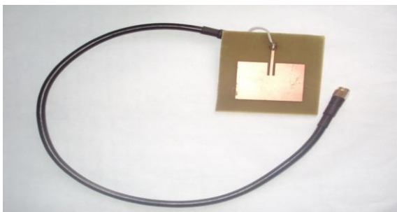
Figure 11. Fabricated RMSA with Inset Line Feed
