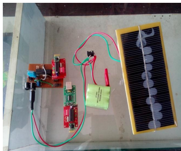
Fig.1 Solar powered wireless sensor
