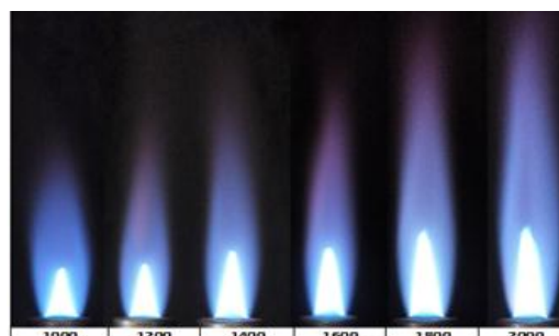
Fig.3. Flame shapes at \phi=1.2 and at Re=1000, 1200, 1400, 1600, 1800 and 2000 .
